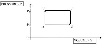
**9**. The figure shows a thermodynamic cycle adcda which a gas may be taken starting at a. Temperatures are: At a T=300K; at b and d T=600K and at c T=1200K. At a the pressure is 100kPa and the volume of the gas is  $1.0m^{3}$ .
